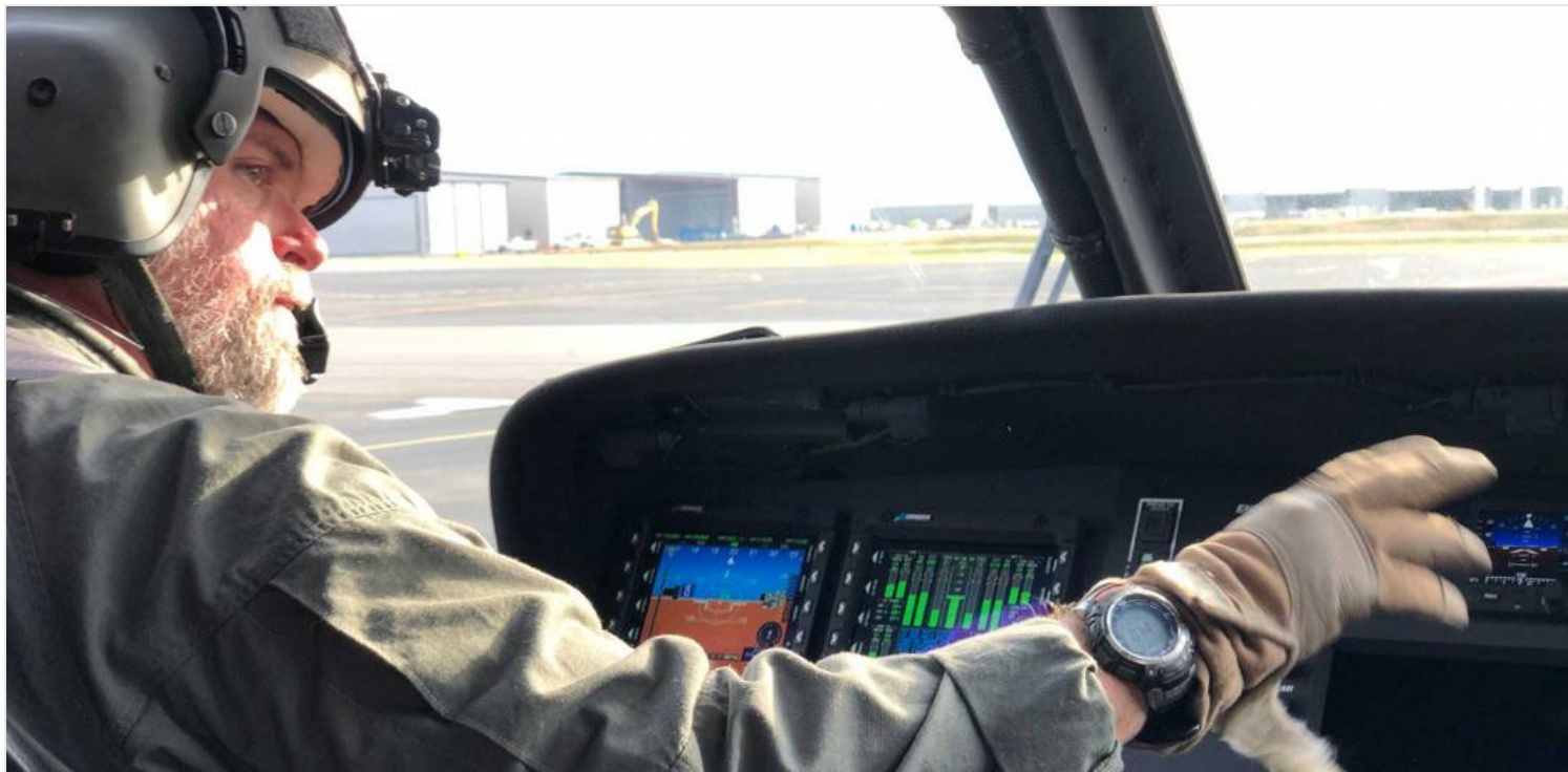
XP Services test pilot Thad King demonstrating the features of the Genesys HeliSAS.
