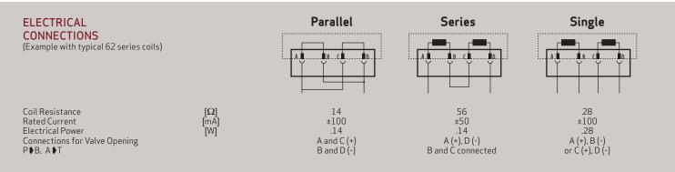
$Note: Before\ applying\ electrical\ signals, the\ pilot\ stage\ has\ to\ be\ pressurized.$
