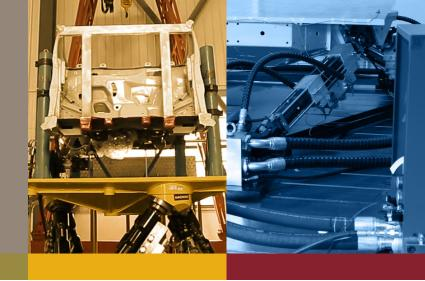
Moog Hydraulic Simulation Table (HST) is a dynamic system, designed to perform research and development tests. The hexapod configuration used by Moog HST is the optimum design to achieve simulation and test capability using acceleration, force, and displacement inputs, and to reproduce data collected on proving grounds regardless of your test type, method, or specimen.
