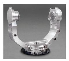
The DSG system provides inertial stabilization of a sighting system for reconnaissance, target acquisition, tracking and engagement. The TRL 8 system consists of a two-axis electro-mechanical yoke paired with Moog's MC100D dual axis motor controller, and is designed for compatibility with several sighting systems currently in USG inventory. The gimbal includes servo driven brushless DC
