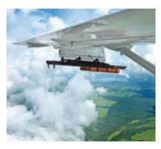
The Moog Missile Simulator (MSL SIM) is a flightworthy, rail-mount design that simulates different types of AGM-114 HELLFIRE® missiles. It can inject faults, provide detailed status, and generate log files for analysis. Available as a simple, pre-configured Captive Air Training Missile (CATM) replacement, or as a full-featured test and diagnostic asset, the MSL SIM can be used for in-flight training, maintenance operational checks (MOCs), and software development.
