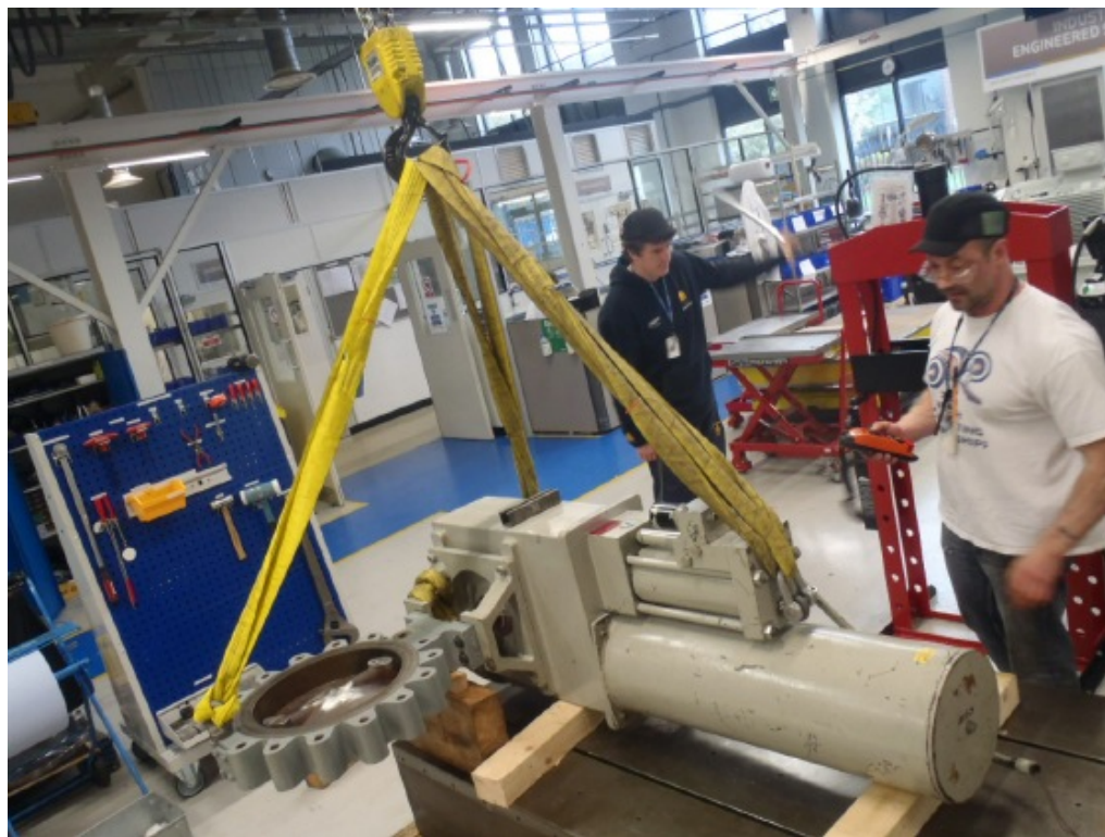
Moog technicians positioning actuator for disassembly
