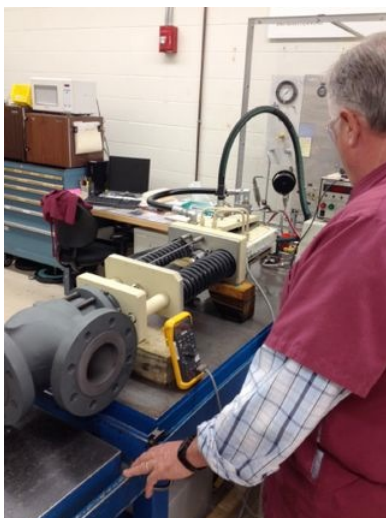
Moog Gas Turbine Actuator being tested after overhaul
