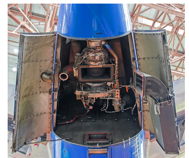
Auxilliary Power Unit
