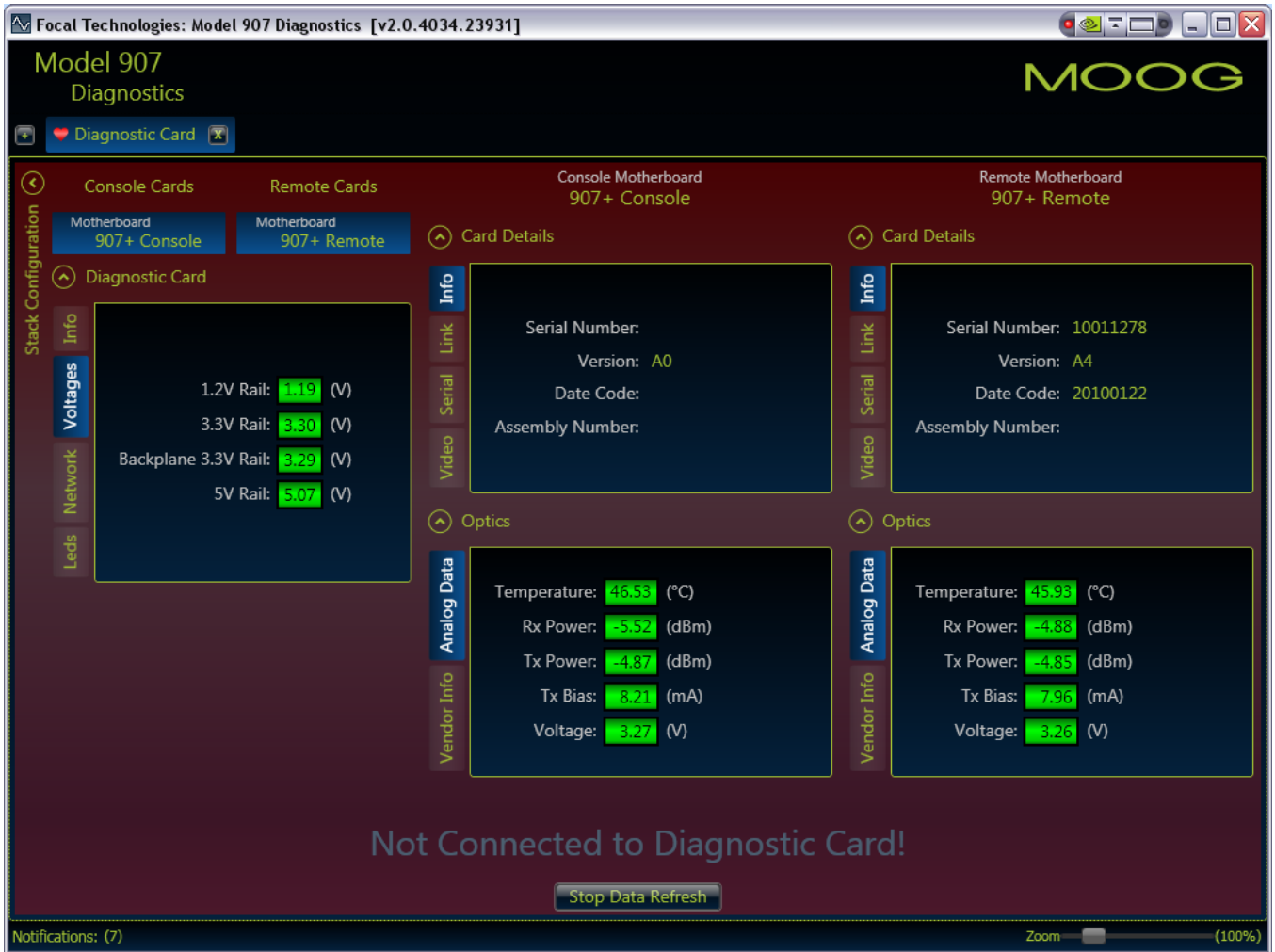
Figure 3-6: Connection Status – “Not Connected” Overlay
