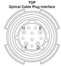
Front face of the optical cable plug pin insert shown. Transceiver insert opposite.
