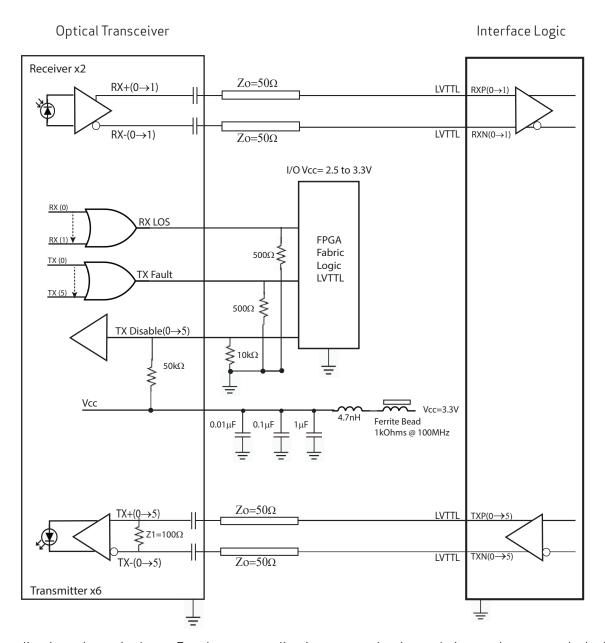
Typical application schematic shown. For alternate applications or termination techniques, please consult the factory.
