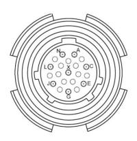
Front face of the optical cable plug pin insert shown. Transceiver insert oppostie.
