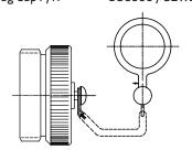
\*CABLE BACKSHELL MIL-C-85049 CABLE BACKSHELL
