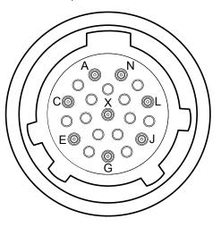
Front view of the D38999 optical insert shown, fiber optic cable plug opposite - see Appendix A1 for details.
