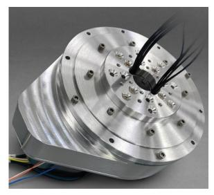
The small SADA is a lightweight and compact power solution for positioning solar array panels. It is comprised of modular components, allowing modifications to meet mission specific requirements. Moog leveraged new design and manufacturing design processes to enable a lighter product with reduced lead times.
