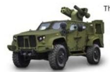
The European designed and manufactured FMP is a missile and platform agnostic system which allows users to seamlessly integrate weapons, sensors, or other assignment packages onto any required vehicle, container, or trailer. Engineered with adaptability in mind, the FMP is available in either a pedestal or yoke form.
