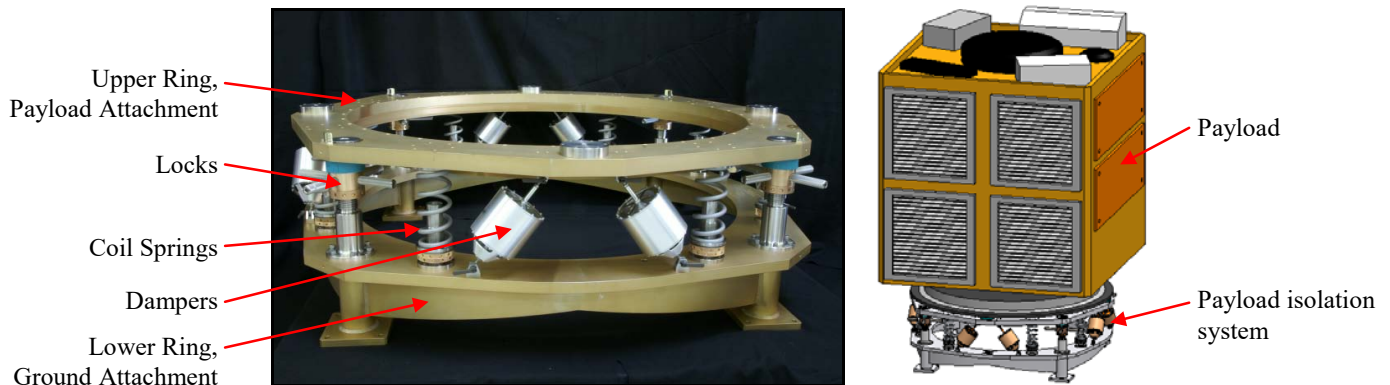
Figure 1. Payload isolation system
