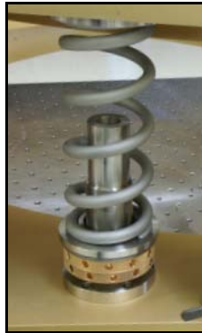
Figure 2: Spring and spring height adjuster
