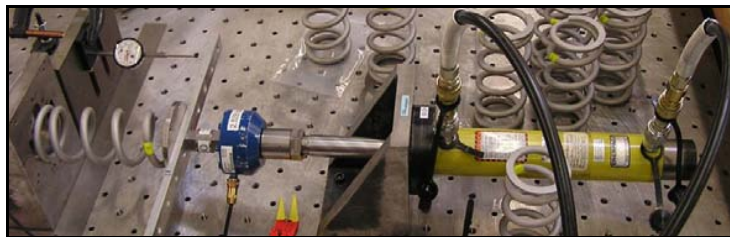
Figure 8: Spring stiffness testing
